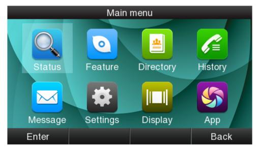
Move the cursor via navigation key and press the softkey "**Enter**" or input the corresponding Number key Select the item of Main Menu:
